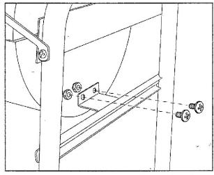
Install smokestack bracket (item #18) into grill lid (item #17 using two M6 x 15mm Phillips head bolts and M6 hex nuts.
